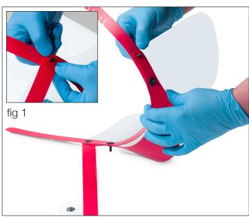
7: Take the visor peak and locate it over the bolt and clear visor. Push on the retaining nut and secure the first hole. Take the remaining bolt and insert it through the last hole of the head strap and visor. Bring across the secondary head strap and push it over the bolt as shown (fig 1). Add the remaining nut to secure all the pieces and push together to fix.
